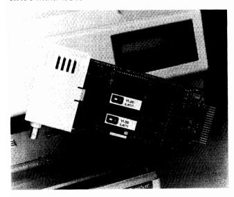
Now you can penetrate the \$1.3 billion IBM 3270 printer marketplace with the HP LaserJet Series II printer. Local Data, Inc., recently announced NEWPORT, a miniaturized protocol converter that plugs into the HP LaserJet printer to provide direct connection to IBM mainframe systems.
