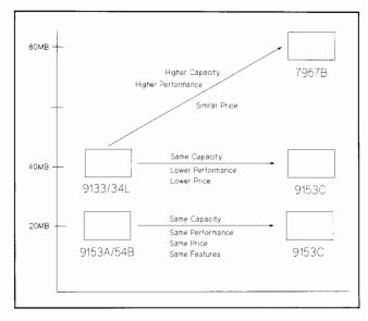
The 20-Mbyte version of the HP 9153C has the same capacity, performance, and price as the HP 9153A/54B disc drives but provides almost doubled microfloppy capacity and improved reliability. Those customers requiring more data-storage capacity will now have the option to prioritize price and performance.
